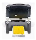
\* Not all cap drivers will be used with this rack orientation (for example: 8 of the 12 cap drivers will be used for a 96 SBS format rack in portrait orientation)
