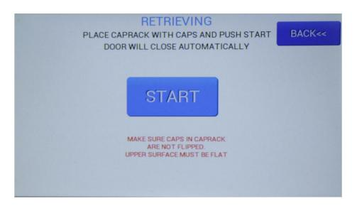
• The device will automatically activate the cap retrieving function.
