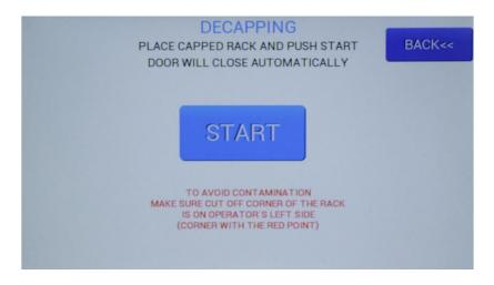
• The device will automatically activate the tube decapping function.
