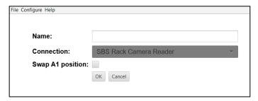
3. Enter a name for the reader and if more than one reader is connected; select the reader from the *Connection* drop down menu
